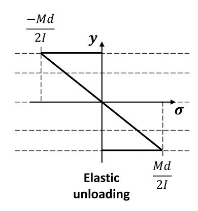
This residual stress distribution will be accompanied by a residual radius of curvature, which can be calculated by substituting unloaded beam values for y and  $\sigma$  into the expression derived for R, which again relate to a position that has only been subjected to elastic behaviour.
