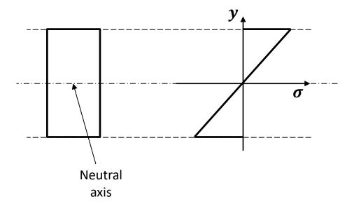
If the bending moment is increased to a magnitude which is just high enough to induce plasticity within the beam, this plasticity will occur at the positions furthest away from the neutral axis, i.e., at the positions of maximum y magnitude (top and bottom edges of the cross-section).
